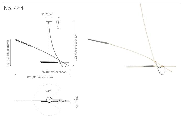
The OTTO Two Arm features two arms extending from a drop. The naturally occurring arcs of the fixture will vary depending on the length of the drop. The OTTO shade contains a dimmable LED source and rotates 300° to cast light directionally. The fixture can rotate 245° from the canopy.
