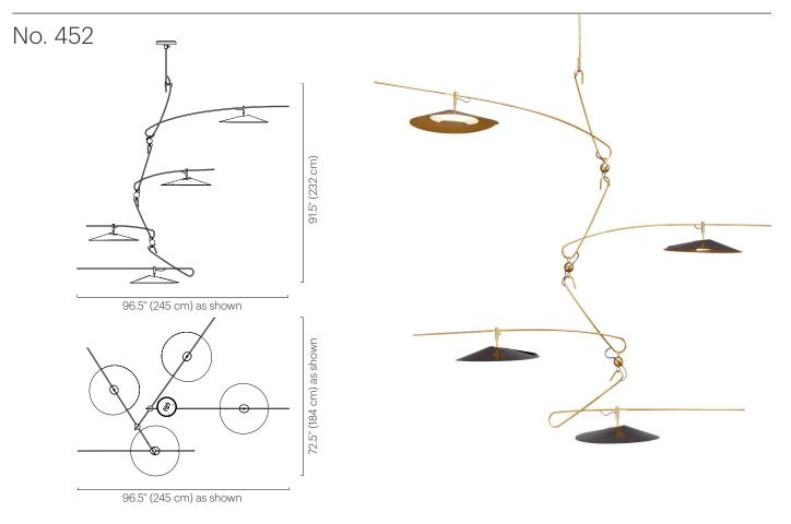
The Treble Mobile features four tiers of different lengths that balance on asymmetrical axes, which allows gentle movement. Each tier has one Treble shade constructed from a flat cut aluminum pattern held together in tension, illuminated by a dimmable LED with a glass diffuser. The fixture can rotate 245° from the canopy. Tier rotation is adjustable and can be set on site.
