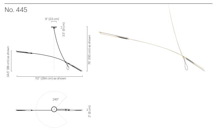
The OTTO Double features one arm with a shade on either end extending from a customizable drop. The naturally occurring arcs of the fixture will vary depending on the length of the drop. The OTTO shades contain a dimmable LED source and rotate 300° to cast light directionally. The fixture can rotate 245° from the canopy.
