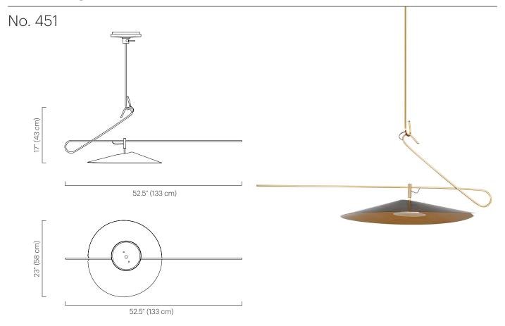
The Treble Single is a balanced fixture on an asymmetrical axis, which allows gentle movement. The fixture has one Treble shade constructed from a flat cut aluminum pattern held together in tension, illuminated by a dimmable LED with a glass diffuser. The fixture can rotate 245° from the canopy.
